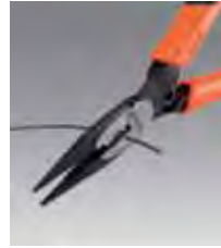
Snipe nose pliers are also used for assembly work. The slender jaws make the work easier in confined spaces.
