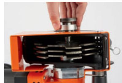
Effortless tool change thanks to split safe-spindle and precision-fit spacer rings
