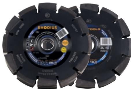
The ALL IN ONE enables quick and operator-friendly chasing of wall slots in a wide variety of materials. Thanks to the ingenious system, using segments arranged in a criss-cross formation, precise wall chasing is now possible, whereby all of the material is removed cleanly from the groove. No time-consuming chiselling out of the middle channel is required. The high-performance, laser-welded ALL IN ONE disc system cuts aggressively and features a long lifetime.
